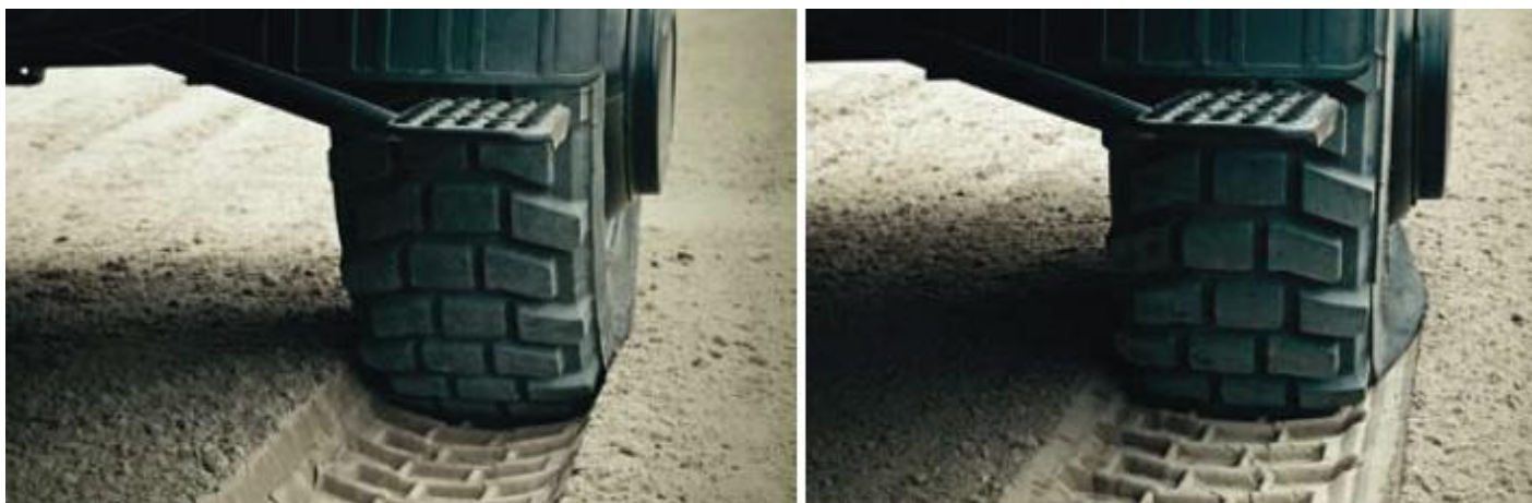
Fig 1 – Mercedes Benz vehicle with CTIS showing effect of decreasing tyre air pressure
