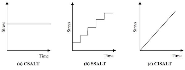
(a) CSALT = Constant Stress Accelerated Life Testing(b) SSALT = Step Stress Accelerated Life Testing
