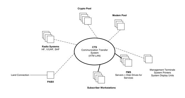
Figure 1 A Typical Communications System Architecture
